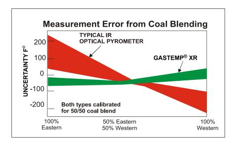
The GASTEMP® XR's design has been proven to be significantly less sensitive to fuel changes than other commercially available devices.
